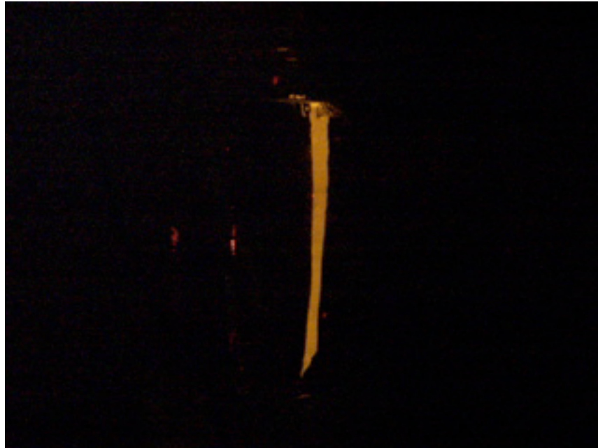
Photo 1 - Orange glow anode 179 V, 3.2 mA
